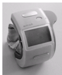
Fig. 3: Prototype AMON wrist-worn device (Anliker, U., et al. , 2004).
