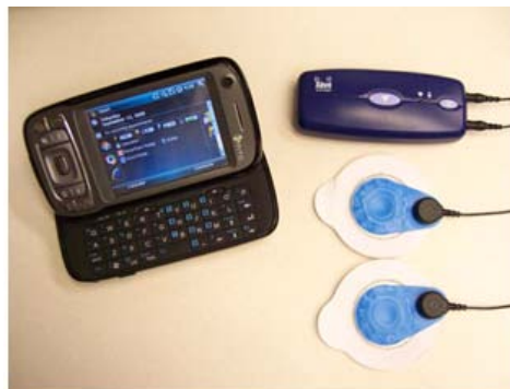
Fig. 7: HeartToGo Platform Prototype, in cooperation with a Microsoft Windows Mobile cell phone with a wearable 2-lead Alive Heart Activity Monitor and a built-in 3-axis accelerometer (Zhanpeng, J., 2009).
